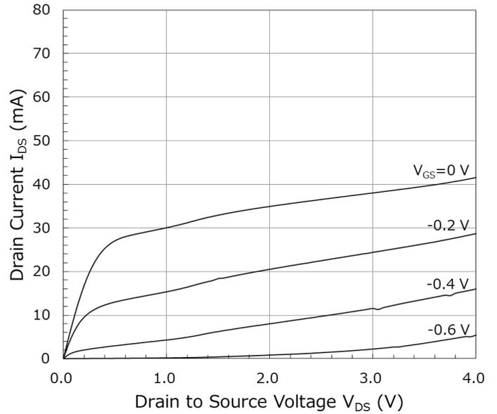
**DRAIN CURRENT vs. GATE TO SOURCE VOLTAGE**
